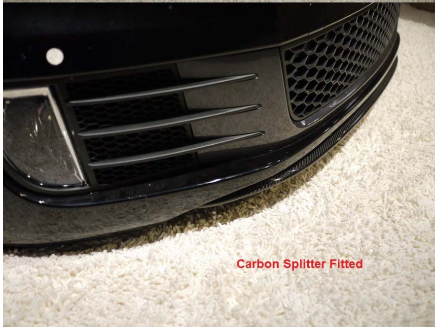
Carbon Splitter Fitted
