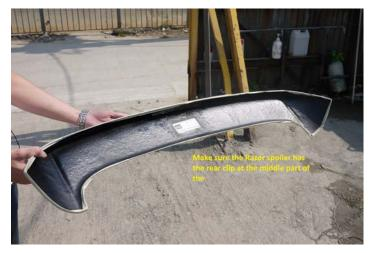
When you received the Razor roof spoiler, please make sure you see a thin black strip at the middle bottom of the spoiler. This piece is to secure the roof spoiler in position.
