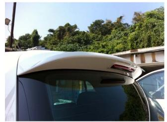
The Razor Roof spoiler is made to clip on top of the original GTi, GTd and R roof spoiler.
