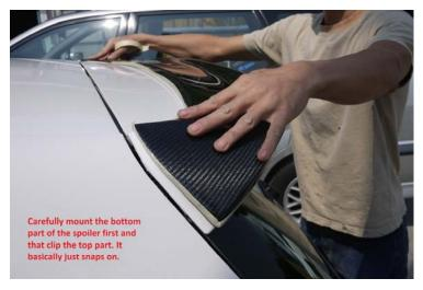
Carefully mount the bottom part of the spoiler first and then clip the top part to towards the end of the original spoiler.
