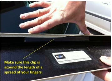
The size of the clip is about the spread of your fingers. There's a slight chance that this clip maybe a bit too long and requires trimming but this is not the usual case. Try to test fit it on your car first and see if the size is right. If not, try trimming it down.
