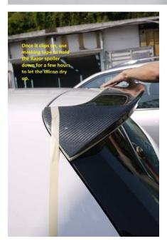
Once it clips on, use masking tape to hold the Razor spoiler down for a few hours and let the silicon dry up.
